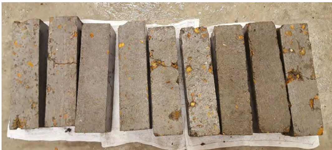
Figure 4.5. RCC specimens after 123 freeze-thaw cycles
