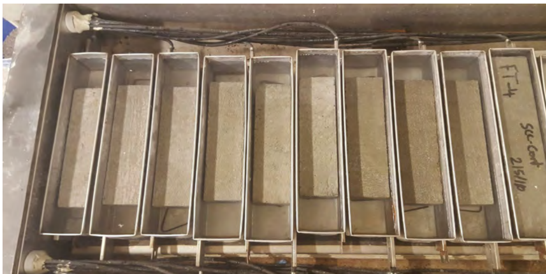
Figure 3.14. RCC specimens before the freeze-thaw test
