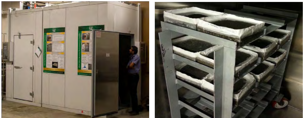
Figure 3.15. Chamber used for deicing salt-scaling resistance test
