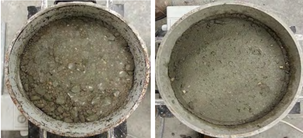
Figure 3.8. Concrete surface after Vebe testing for (a) dry RCC with low workability level (Vebe time \geq 90 s; (b) RCC with medium workability level (Vebe time = 45 s) (Khayat and Libre, 2014)
