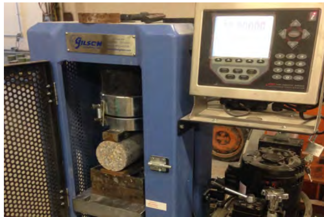
Figure 3.10. Splitting tensile test setup
